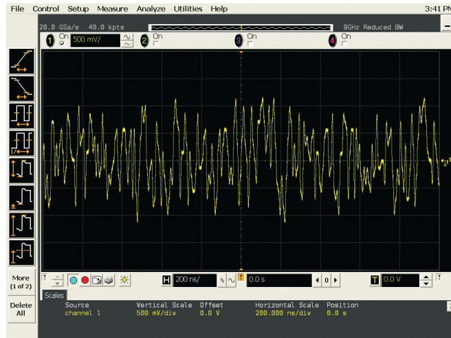
Figure 16. The Test Mode 4 waveform.
