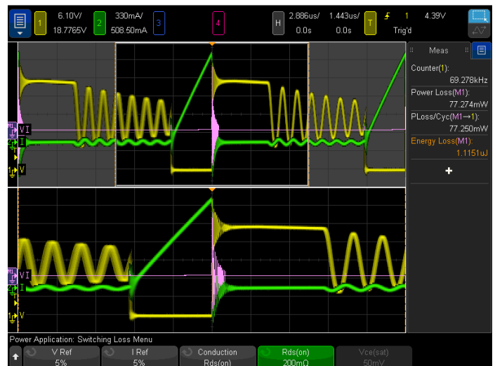
Figure 18. Measuring power and energy losses based on using an entered value of R_{ds(on)} .
