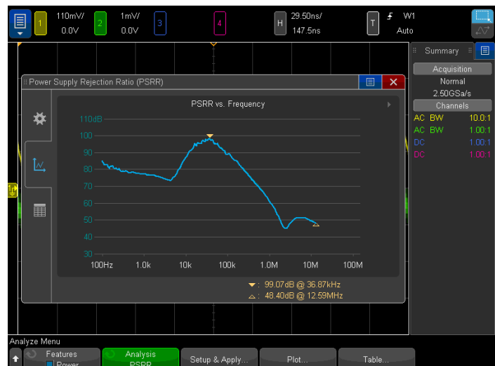
Figure 37. Power supply rejection ratio (PSSR) measurement using the scope's built-in waveform generator as an automatic swept source.
