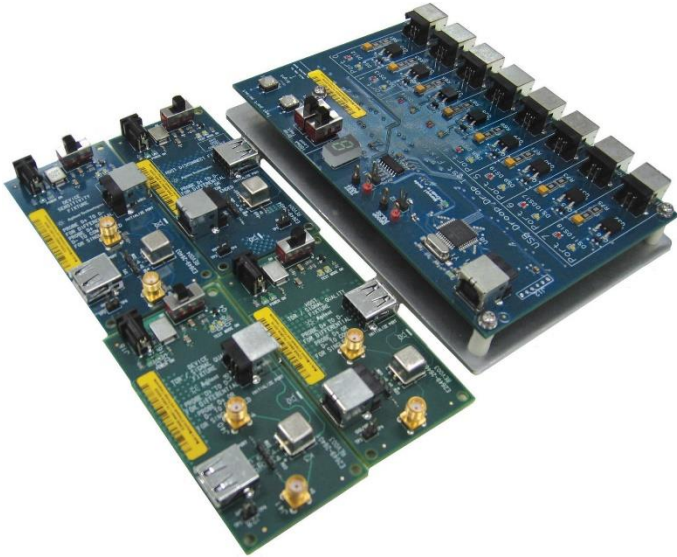
Figure 10. Hi-speed signal quality boards (Keysight fixture and Intel fixture—device signal quality test).
