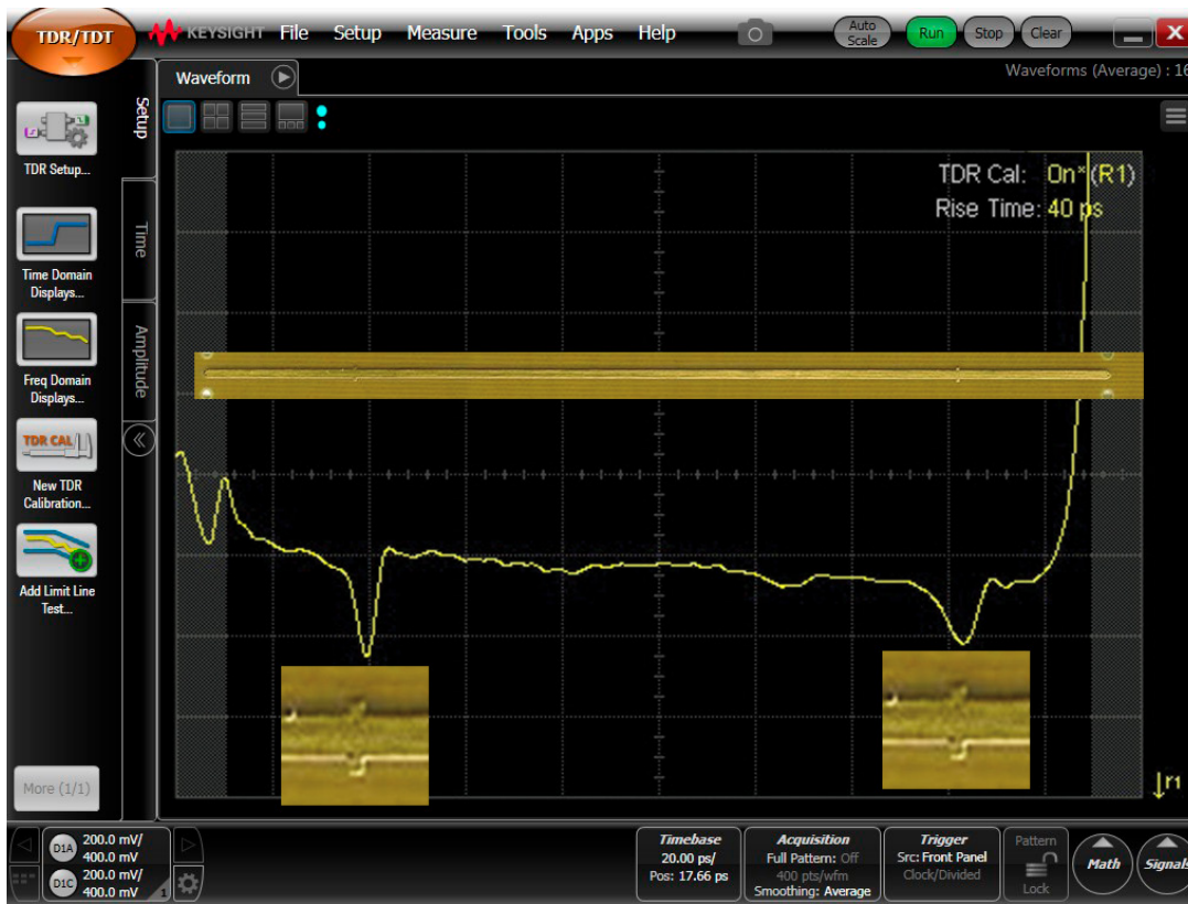
Figure 9. TDR response of a uniform transmission line with two small reference pads, located on four inch centers.
