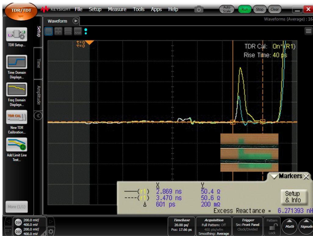
Figure 20. Using markers to extract the excess inductance of a large gap in the return path.
