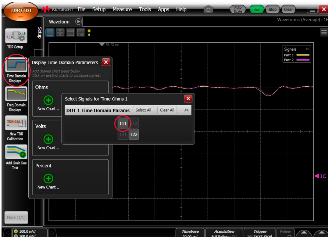
Figure 3. Using the advanced settings function to adjust the vertical scale to display the impedance directly.
