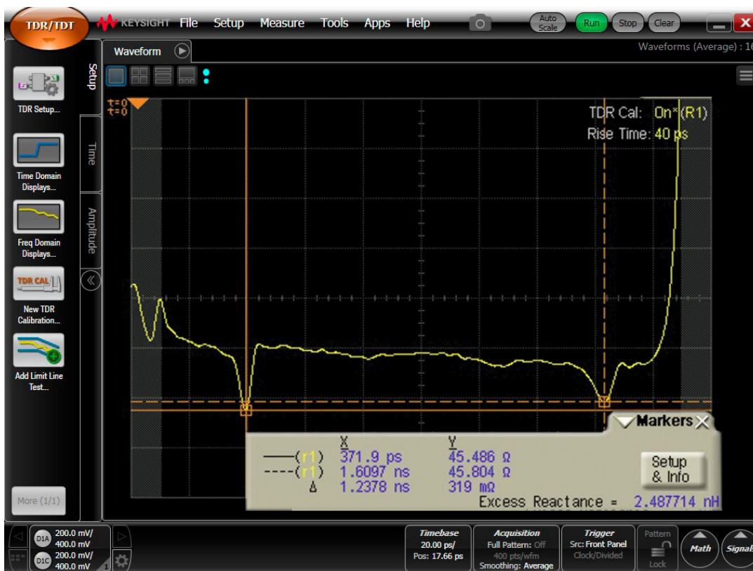
Figure 10. TDR response from a microstrip with two reference pads, using markers to measure the round trip time delay.
