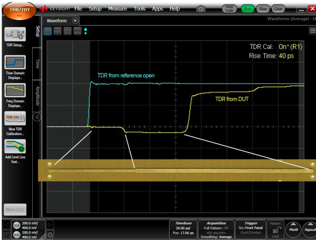
Figure 1. Measured TDR response from a microstrip transmission line. Blue trace is the reflection from the end of the cable; yellow trace is the reflected signal from the DUT.
