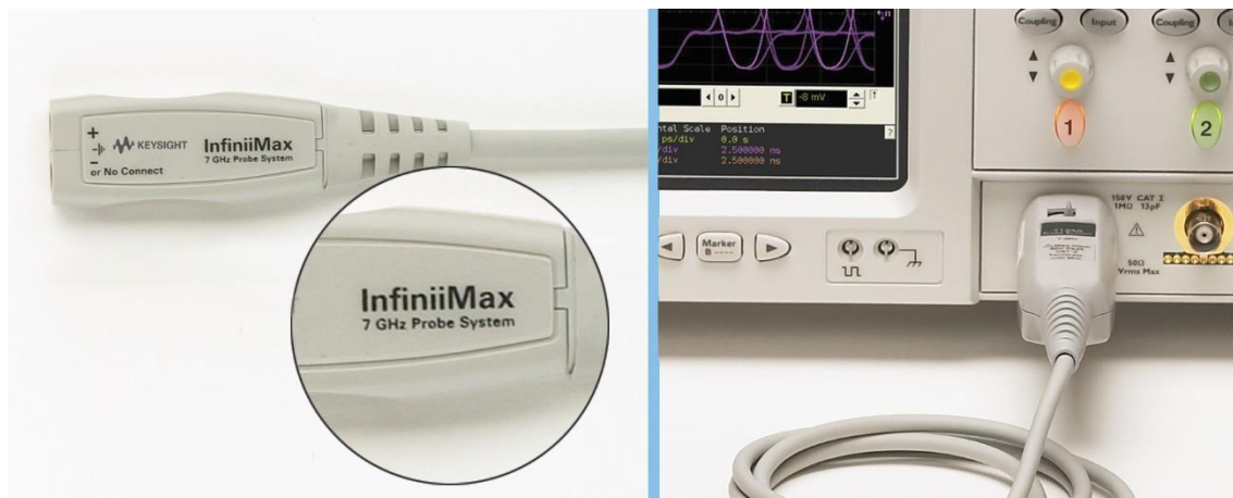
Figure 30. An active probe.
