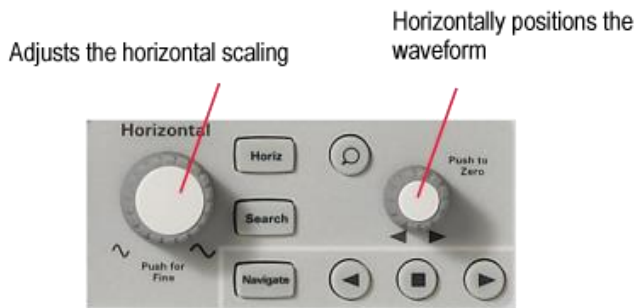
Figure 17. Front panel horizontal control section on a Keysight InfiniiVision 2000 X-Series oscilloscope.
