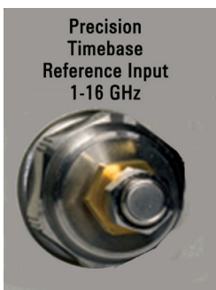
Figure 13. The 86108 Precision timebase reference input
