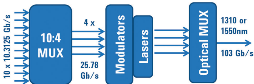
Figure 1b. Example block diagram of high data rate transmitters for 100 Gb/s
