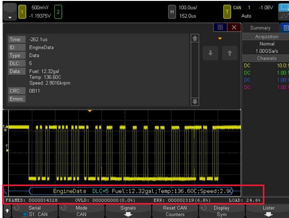
Figure 7. Real-time frame counter and bus utilization measurement helps characterize CAN and FlexRay systems
