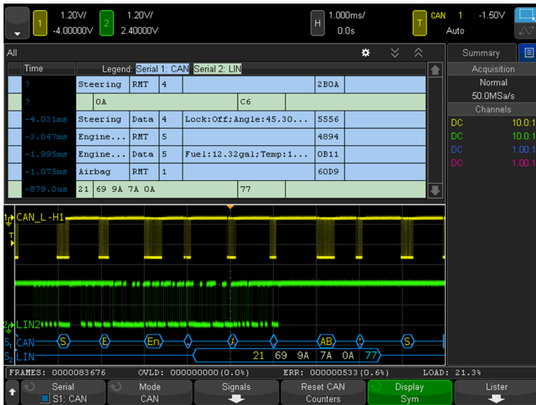
Figure 6. Dual-bus time-interleaved lister display makes it easier to track data through CAN-to-LIN gateways
