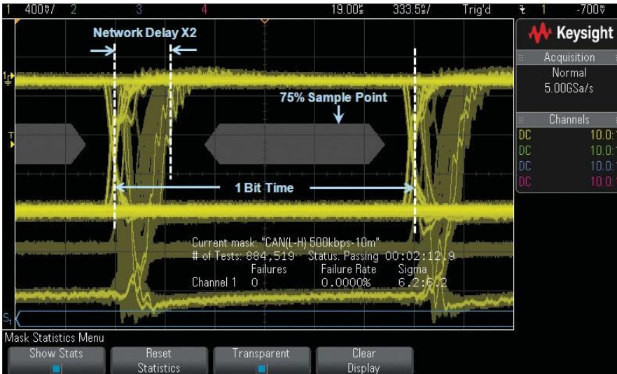
Figure 4. CAN eye-diagram mask testing shows amplitude variations and timing uncertainties, including network propagation delays, from all frames and bits
