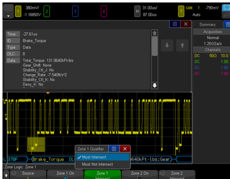
Figure 10. Characterization CAN bus arbitration using the oscilloscope's zone triggering capability
