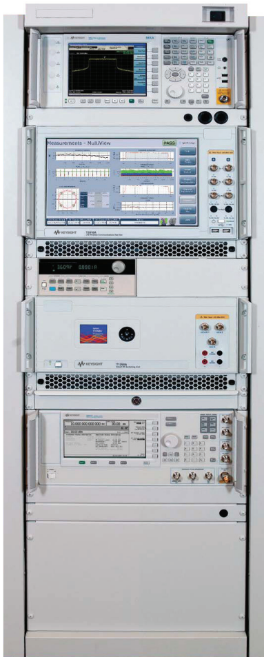
Figure 39. RF conformance test system for LTE UEs
