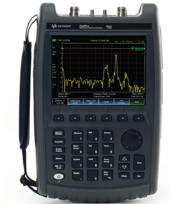
Figure 41. Handheld RF analyzer that combines the functions of six instruments in one integrated, fast, and rugged package
