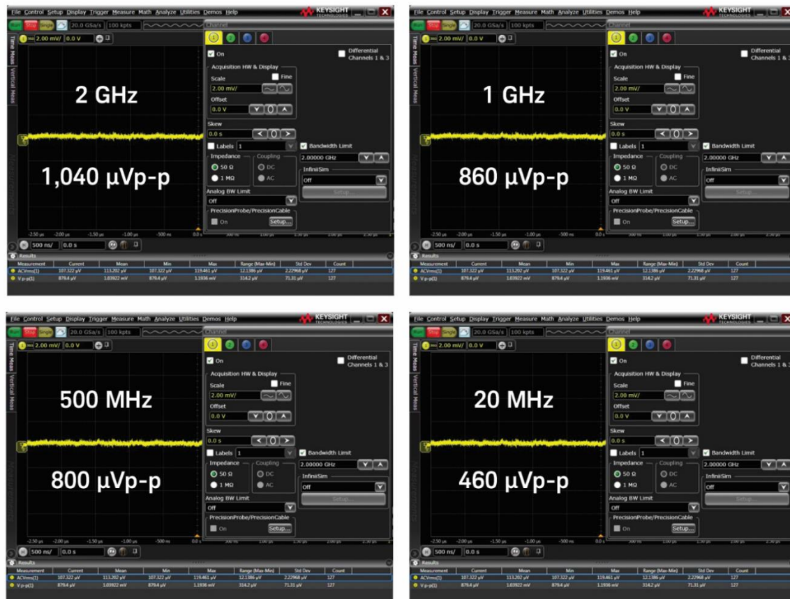
Figure 2. Baseline noise at various bandwidth limits with the Keysight N7020A power rail probe and MXR-Series oscilloscope
