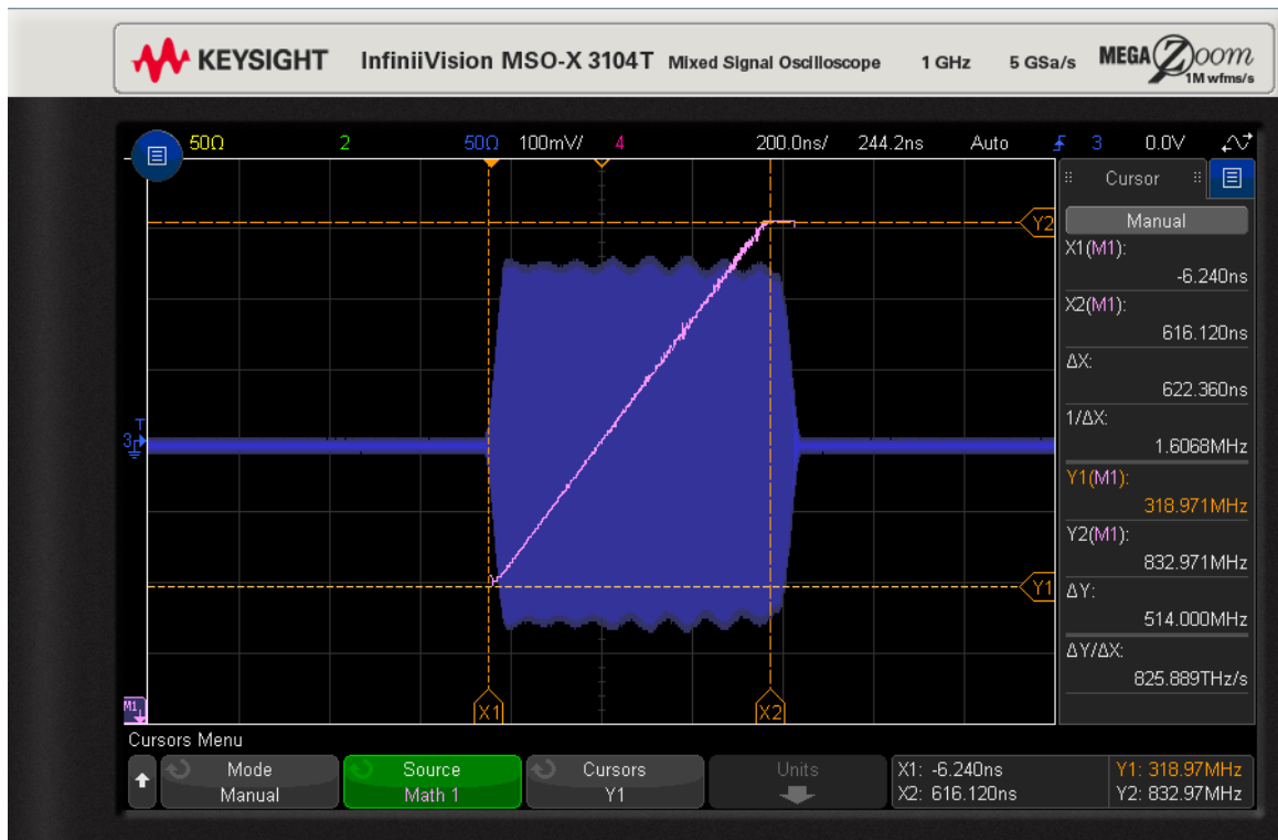
Figure 6. Measurement trend math function on “Frequency” measurements across the pulse
