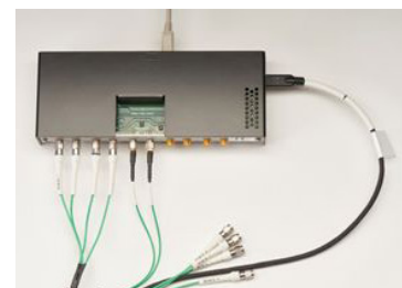
Figure 10. N7016A Type-C low speed signal test fixture.
