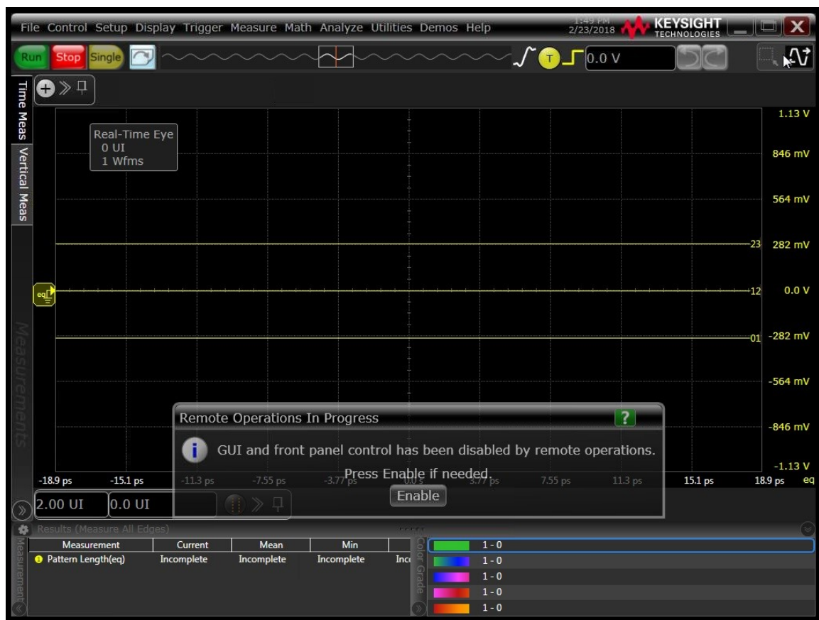
Figure 18. Oscilloscope GUI when remotely controlled from the M8070B
