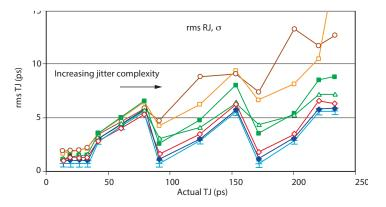
Figure 5: rms RJ measurements by the different test-sets vs the true value of TJ(10–12). The true values of RJ are indicated by the white curve. The error bars on the true values indicate the calibration uncertainty in the calculation of the true values. The complexity of the jitter conditions for each measurement increases from left to right, as does the discord among the analyzers.
