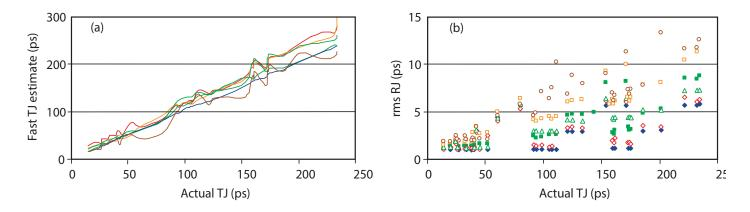
Figure 2: (a) TJ(10-12) estimated by the different test-sets vs the true value of TJ(10-12) and (b) RJ measured by the different test sets vs the true value of TJ(10-12).
