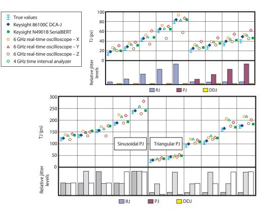
Figure 6: TJ(10–12) estimates with jitter conditions. The jitter conditions (RJ, PJ, DDJ) of each measurement are indicated by the bar graph at the bottom. The true values of TJ(10–12) and the calibration uncertainties associated with them are indicated by the left-most, white, data point in each column.
