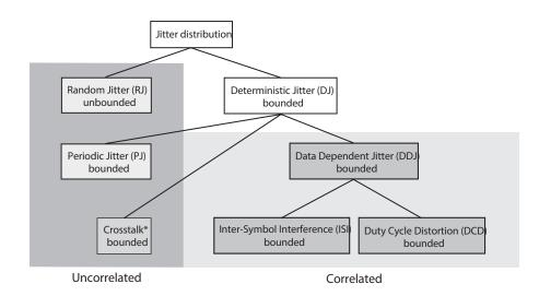
Figure 1: The decomposition of jitter into sub-components. Crosstalk, marked with a \*, is not generally defined and none of the jitter analyzers studied here distinguish it thus its analysis is beyond the scope of our study. Generally, crosstalk can have jitter-like effects but should be analyzed as amplitude noise, not jitter; we include it in this figure for completeness.
