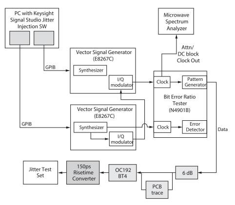
Figure 3: Block diagram of the precision jitter transmitter.
