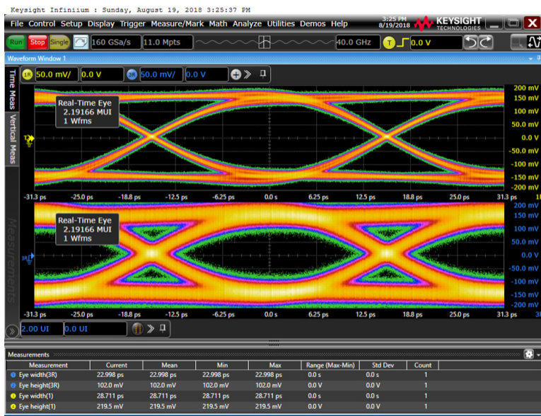
Figure 3: Compared to the clean eye diagram of the direct signal (top), the effects of noise are evident in the lower trace
