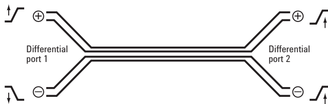
Figure 20: Mixed mode S parameters: S_{CD21} .
