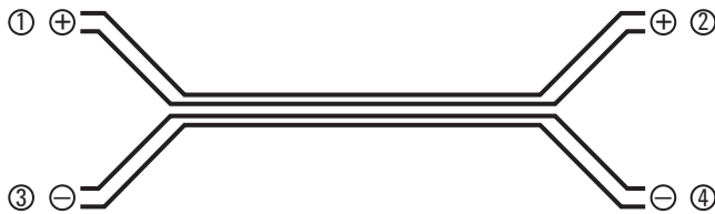
Figure 17: Single-ended S-parameters for a 2 port differential device.
