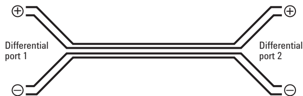
Figure 10. Differential line model.
