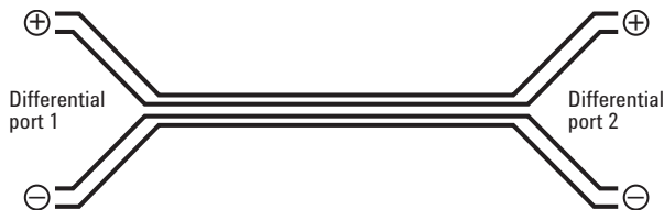
Figure 18: Differential S-parameter model.
