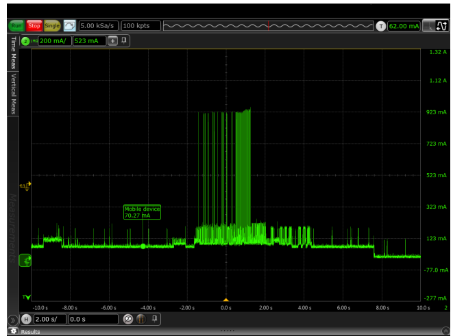
Figure 3. A mobile device requires vertical oscilloscope scaling of 200 mA/div or 1.6 A full screen to capture the high power modes as well as the low-power modes. Oscilloscope resolution in this example equals 1.6 A divided by the number of quantization levels the scope's ADC provides.
