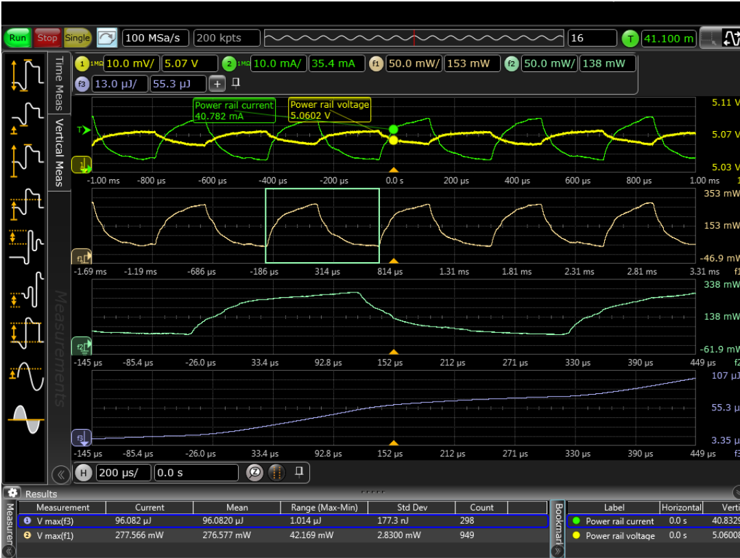
Figure 9. Keysight's Infiniium S-Series provides math, gating, and measurements to report low-power measurement in the correct unit designation values such as watts, joules, and coulombs. This figure shows a low-power USB power measurement. Channel 1 was connected to the power rail for voltage measurements while channel 2 provides a current measurement on the power rail. Power, energy, and charge measurement results have been set uniquely for the designated gated regions.
