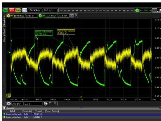
Same signal with BW limiting of 20 MHz
