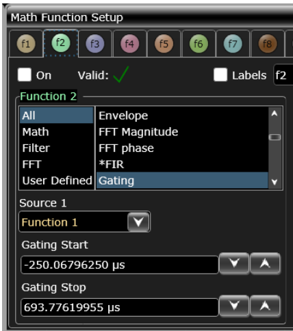
Figure 8. Infiniium S-Series offer measurement gating or any region specified, by using one of the available 16 math functions as a gate. Measurements and analysis can be made uniquely on each gated region. In the example above a gate has been applied to the orange waveform. The gated region is shown in green.
