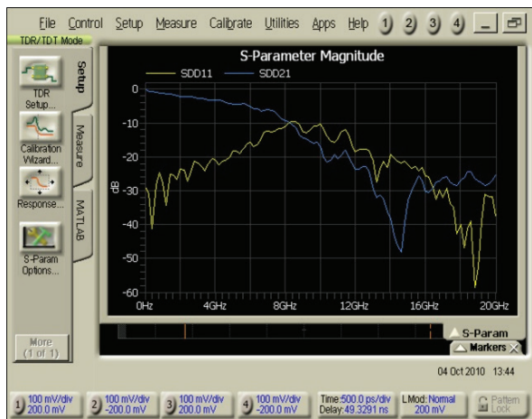
Figure 9. Return loss (SDD11) and insertion loss (SDD21) for Channel A as measured by 86100D Option 202 Enhanced Impedance and S-parameter software.
