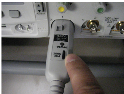
Figure 2. To improve current probe's accuracy remove magnetism and DC offset.
