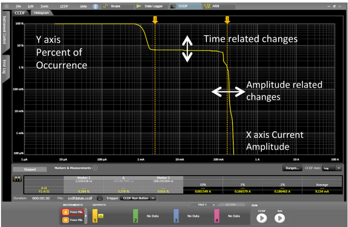
Figure 8. This CCDF measurement reveals the key attributes of standby current in a smartphone.
