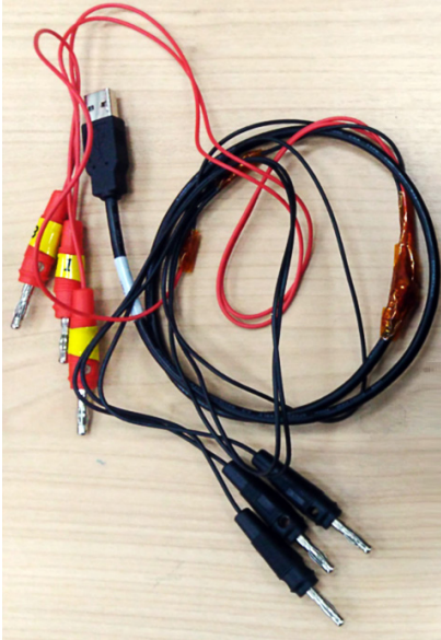
Cable kit to connect the DUT to N6705B/C
