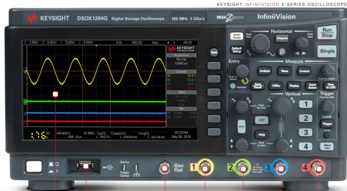
Waveform display area shows waveforms graphically, typically in volts (vertical axis) versus time (horizontal axis). The display area is divided into "divisions" using vertical and horizontal grid lines.
