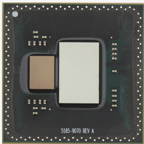
Figure 2. While most oscilloscopes incorporate an 8-bit ADC, S-Series oscilloscopes include a 40 GSa/s, 10-bit ADC. This results in four times the resolution versus 8-bit oscilloscopes.
