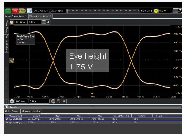
Figure 1. Two Keysight oscilloscopes tested at equal bandwidths show they have very different signal integrity. Here we show an eye diagram from the same source on two scopes each rated at 4 GHz. The Infiniium S-Series shows (right) a more representative eye shape and has an eye height measurement 200 mV higher than what the DSO9404A shows (left). The lower value and more representative shape seen on the S-Series is a result of superior signal integrity.
