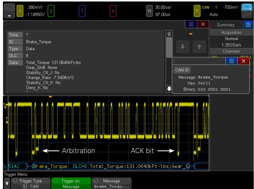
Figure 2. Viewing evidence of arbitration on an oscilloscope.
