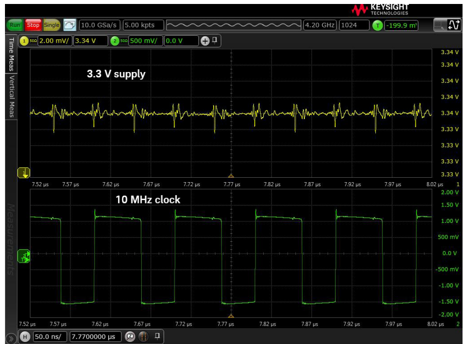
Figure 11. Triggering on the 10 MHz clock and enabling averaging removes all random noise and signals that are not coherent with the clock. The resulting view is of the noise on the supply that is related to the 10 MHz clock.
