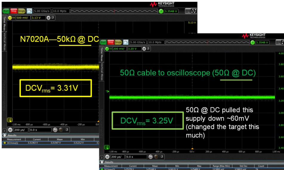
Figure 7. The effects of probe loading on a supply. A 3.3 V supply probed with the N7020A power rail probe with its 50 k \Omega impedance at DC and the same supply probed by direct connection to the 50 \Omega input of the scope.
