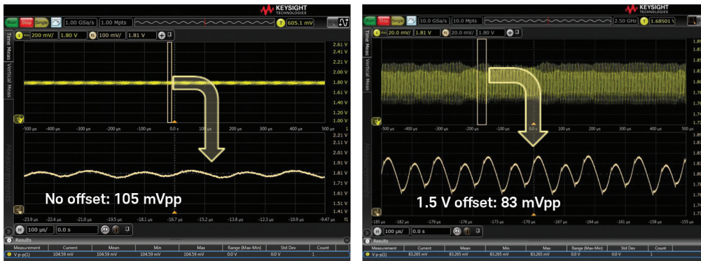
Figure 4. Measuring the noise on a 1.5 V DC supply with no offset and with the use of probe offset.
