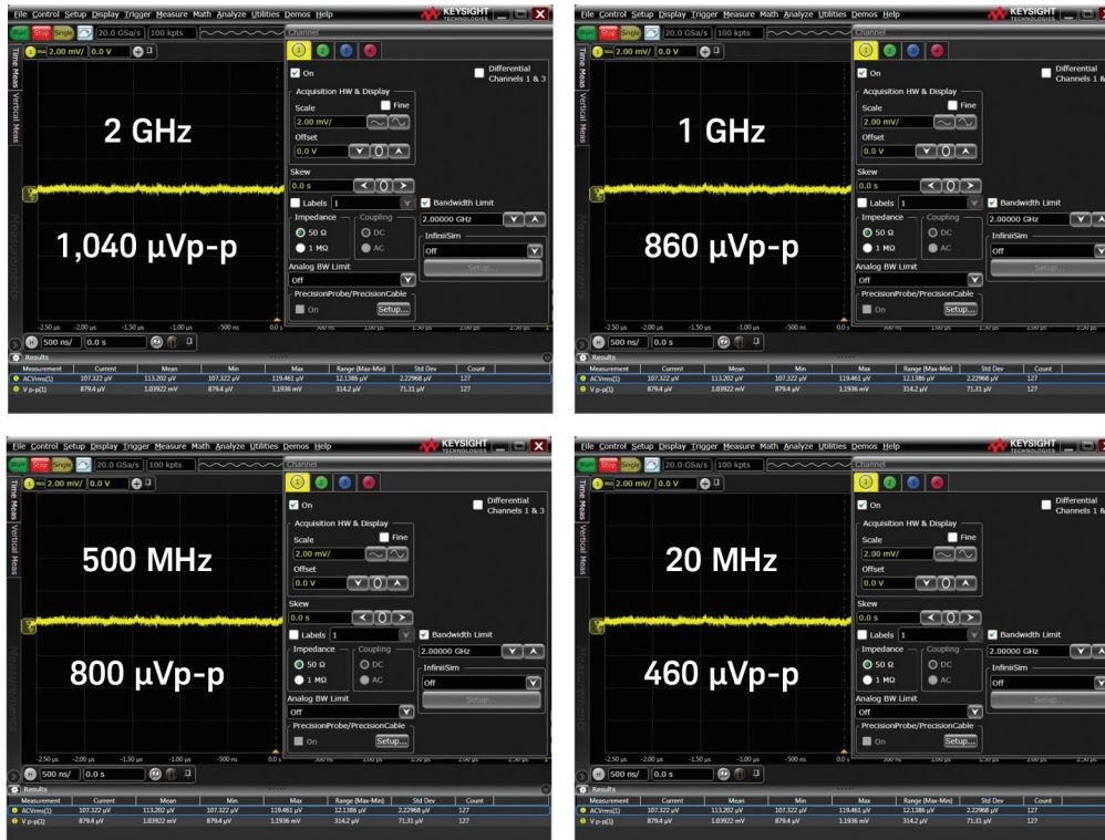
Figure 2. Baseline noise at various bandwidth limits with the N7020A power rail probe and MXR-Series oscilloscope.
