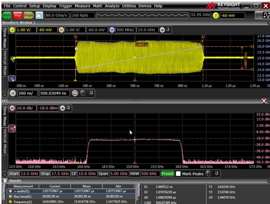
Figure 11. FFT set to a 15 GHz center frequency and to a 5 GHz frequency span.
