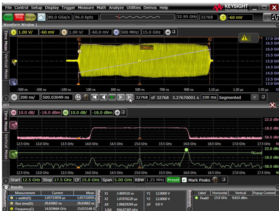
Figure 18. V-Series segmented memory capture of 32k pulses into 32k segments, 1.2 usec per segment.
