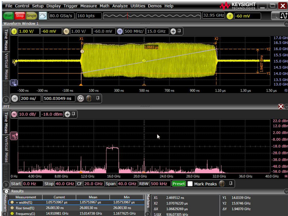
Figure 10. Wideband FFT measurement on 15 GHz carrier, 2 GHz wide linear FM chirped RF pulse with V-Series oscilloscope.
