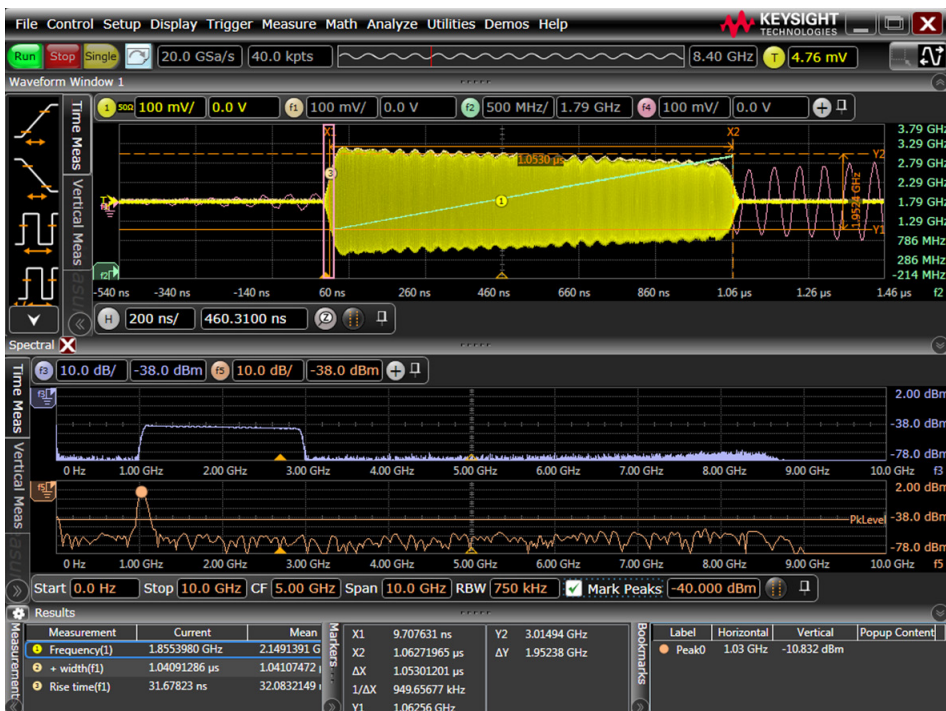
Figure 16. Time domain measurements and FFT on 4 GHz carrier, 2 GHz wide linear FM chirped RF pulse with S-Series oscilloscope.
