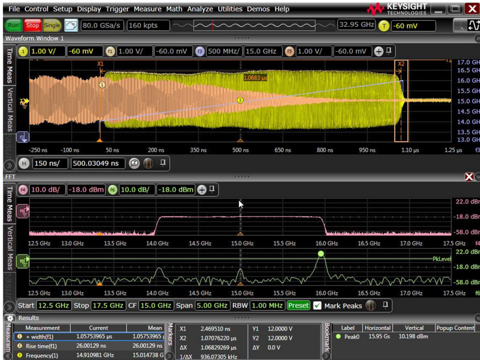
Figure 15. View of time gated FFT and display with time gate at the end of the RF pulse.
