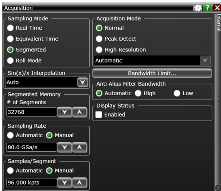
Figure 17. Segmented memory setup to choose 1.2 usec wide segments for 1 usec wide pulse capture.
