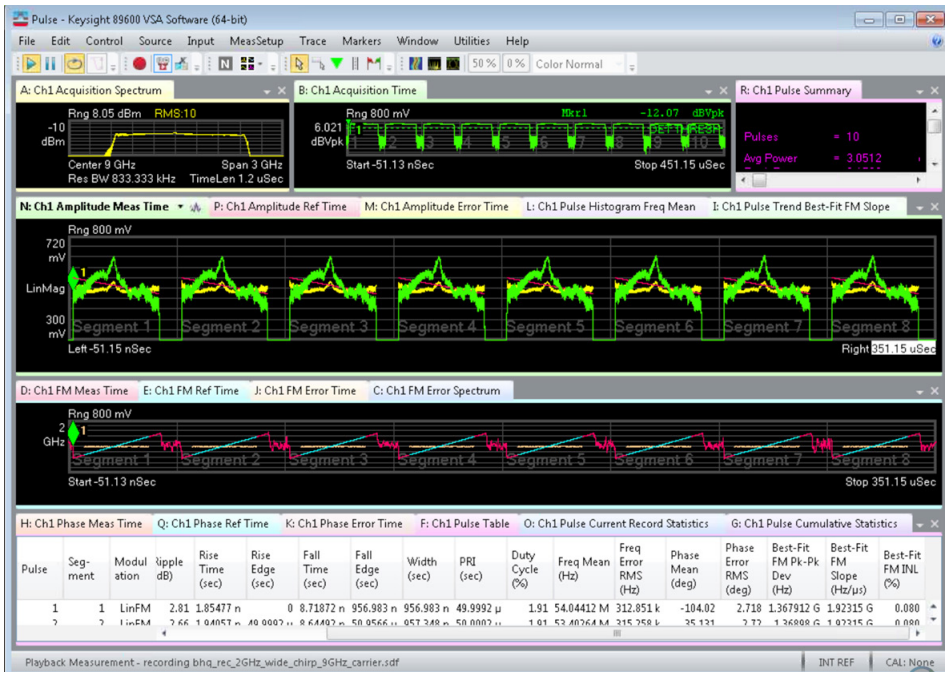
Figure 25. 89600 VSA's pulse analysis option BHQ and pulse parameter measurements on oscilloscope segmented memory.
