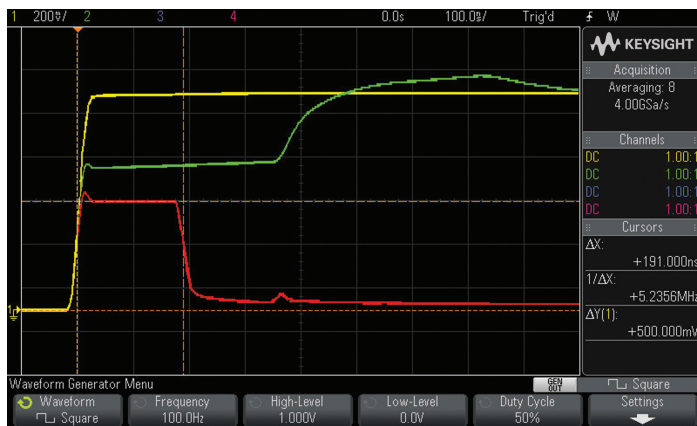
Figure 7. Cable test measurement: without a DUT connected (yellow trace); with twisted wire as the DUT (green trace); with shorted RG-58 as the DUT.
