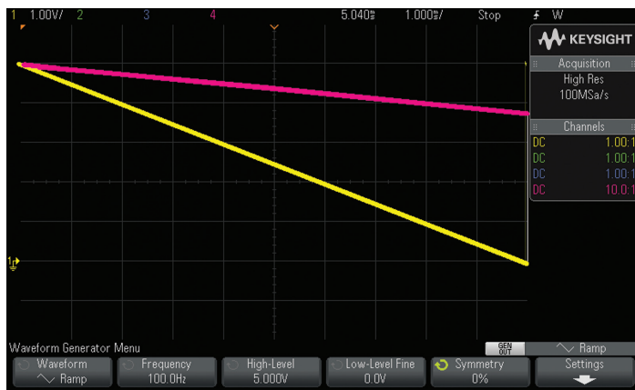
Figure 5. Output resistance measurement: without a DUT connected (yellow trace); with a 74ACT08 DUT attached (red trace).
