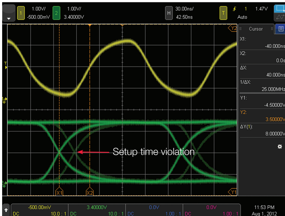
Figure 4. Observing an eye-diagram display of a data signal (green trace) with an occasional setup time violation while triggering on the rising edge of the clock signal (yellow trace).
