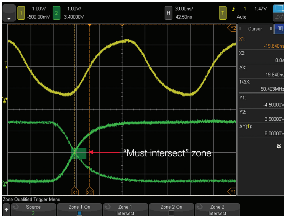
Figure 5. Using Zone Trigger to isolate setup time violations.
