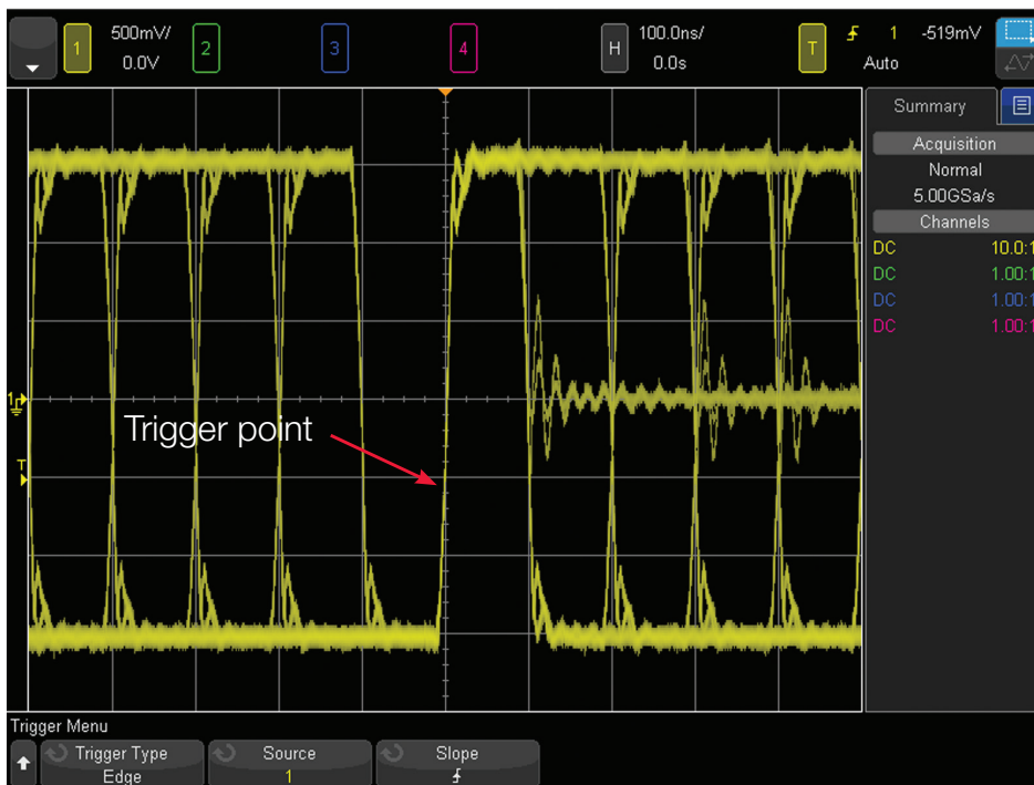
Figure 7. Triggering on a rising edge of a 10 Mbps serial bus signal with the timebase set at 100 ns/div.
