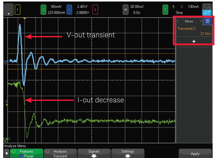
Figure 35. Transient response settling time measurement when output load decreases (output current suddenly decreases).
