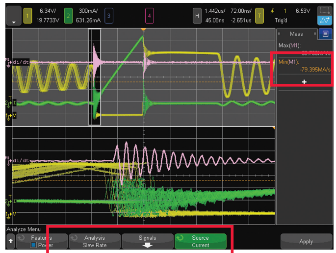
Figure 23. Slew rate measurement of the current waveform during the transistor turn-on phase.
