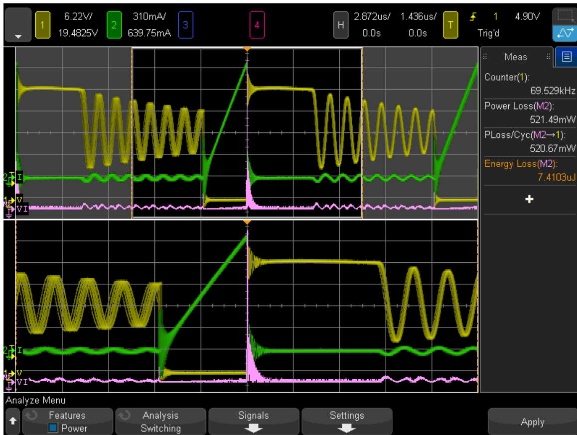
Figure 3. Automatic power and energy switching loss measurement performed by a Keysight oscilloscope
