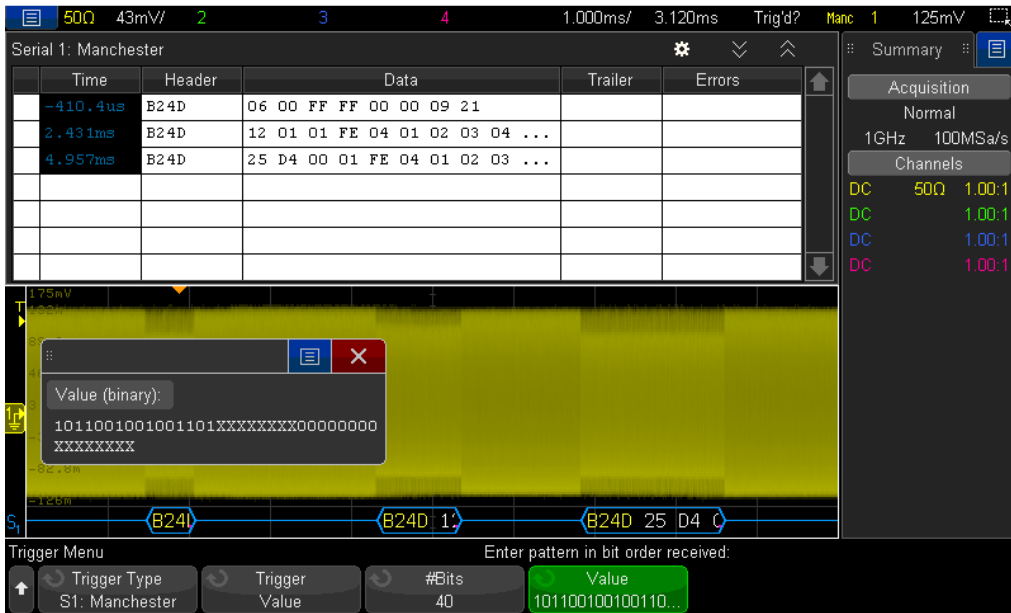
Figure 12. Triggering on SENS_REQ using Manchester triggering.
