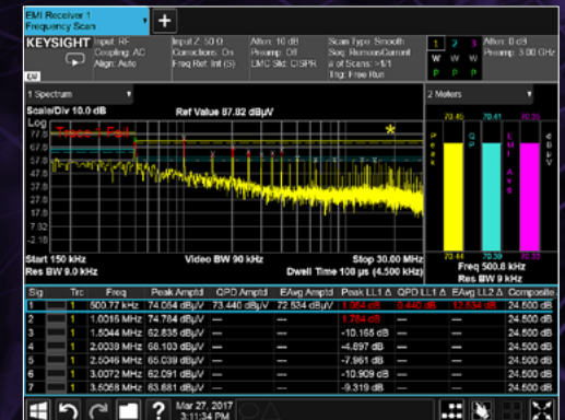
Figure 2.5: When making EMI measurements, you often want to scan and search for signals above the limit.
