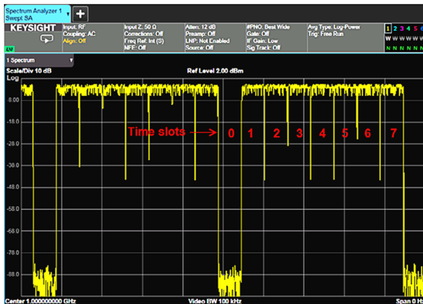
Figure 1.1: A TDMA format signal (in this case, GSM) with 8 time slots; time slot zero is “Off.”
