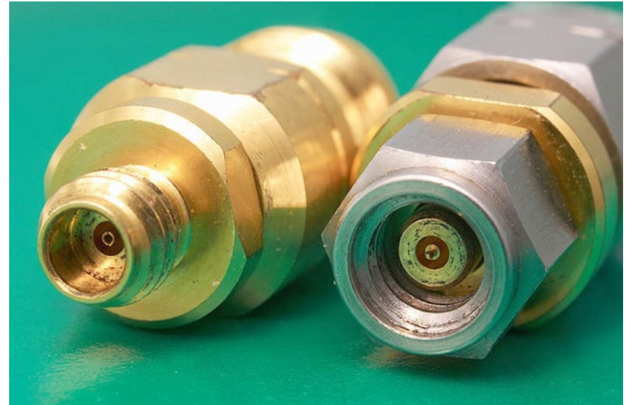
Figure 1. Female and male 1 mm connectors. The center pin in the jack on the right is only one-quarter of 1 mm in diameter.
