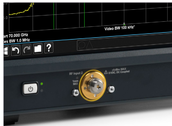
Figure 2. While the typical front-panel connector is female, the gender is often reversed for equipment covering millimeter frequencies (30 GHz to 300 GHz). The male connector offers some degree of protection from several types of damage.
