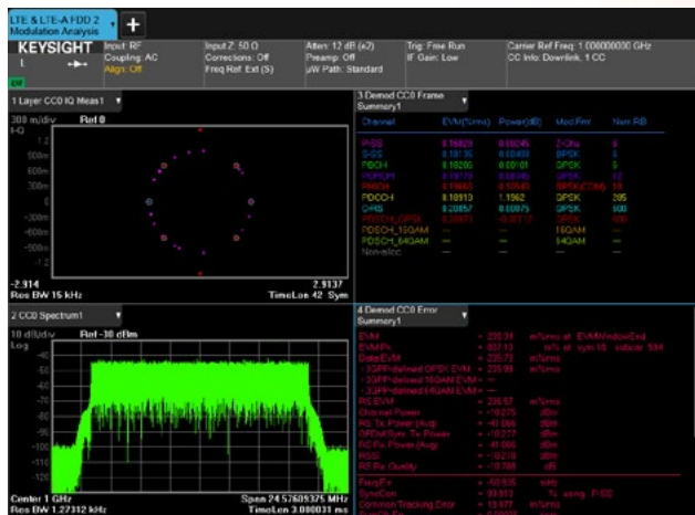
Figure 6. Using the LTE-Advanced FDD measurement application to analyze LTE FDD test model signal quality
