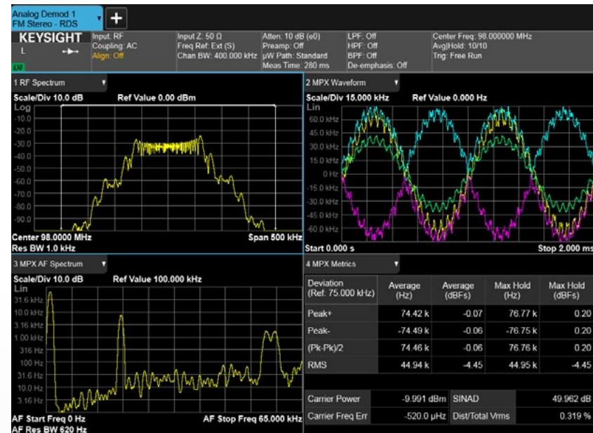
Figure 5. Using an analog demodulation measurement application to analyze the FM Stereo with RDS signal
