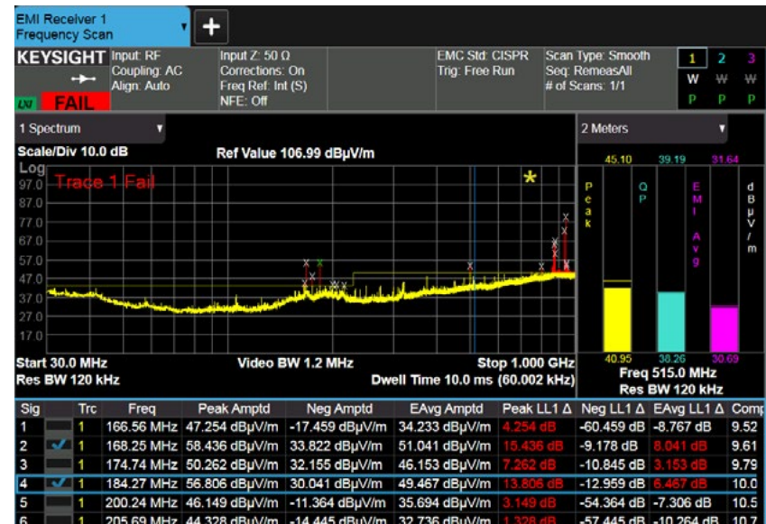
Figure 8. Using the EMI measurement application with frequency scan measurement to make compliance or pre-compliance EMI measurements
